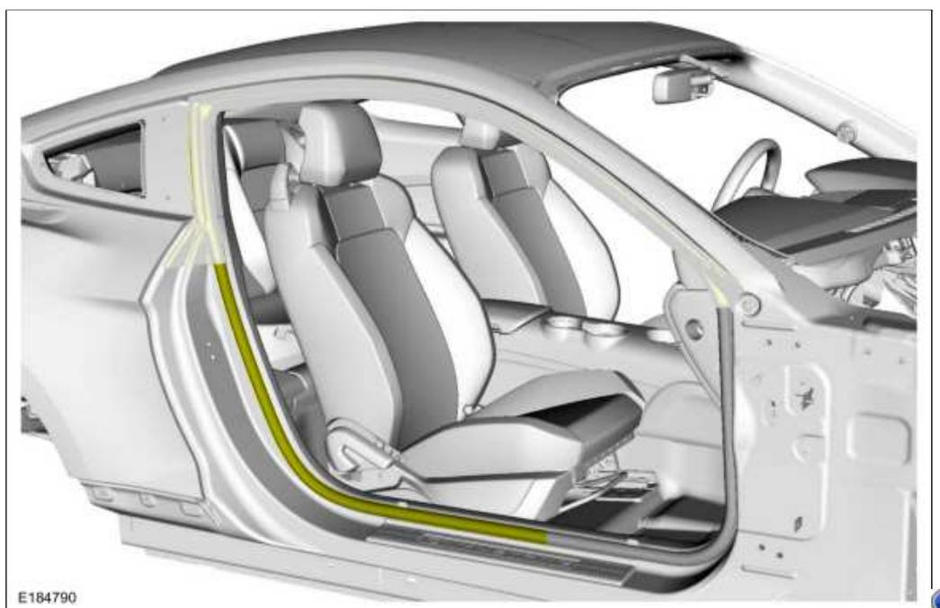
2. Release the clips and remove the scuffplate trim panel.
